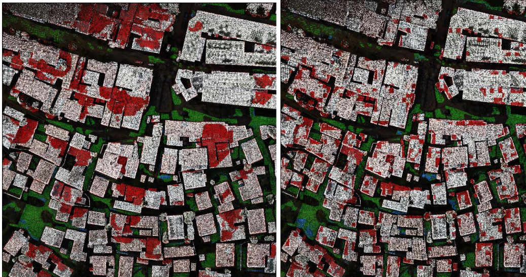
Figure 1. Classification maps showing the accuracy of: the first step to automatically select training labels (a), the final results of the proposed FCN method (b), and two reference DTM extraction methods: gLidar (c) and Lastools (d).
